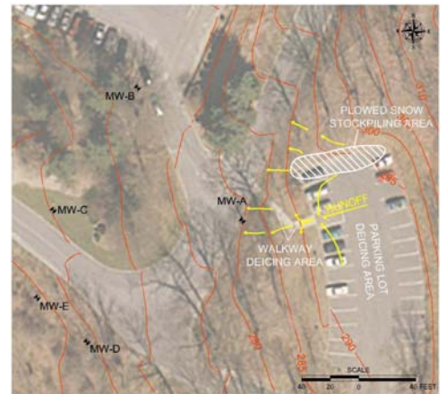
Snow piling, deicing and runoff areas
